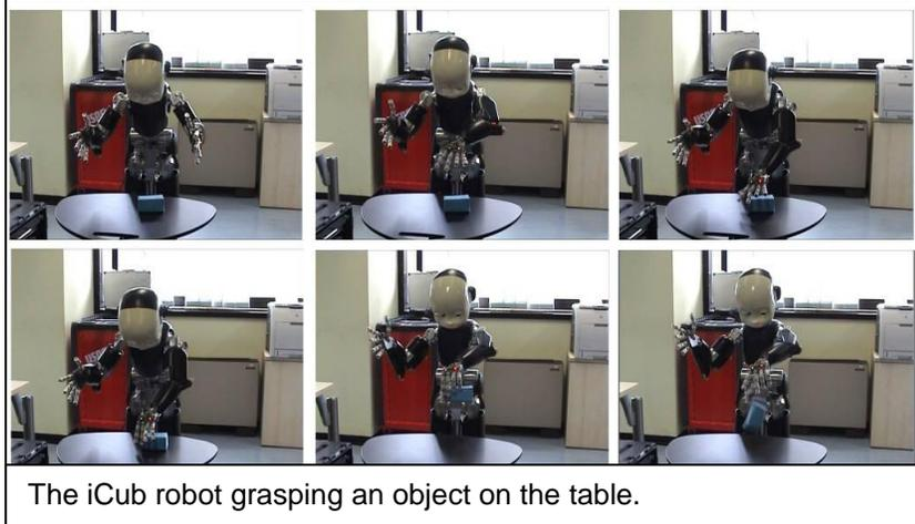
The iCub robot grasping an object on the table.
